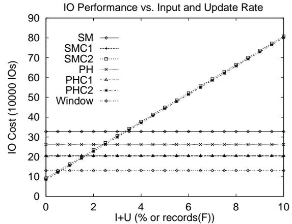
Figure 9: IO Cost and Varying Update and Insertion Rates
