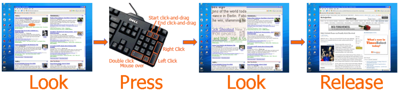
Figure 1. Using EyePoint - progressive refinement of target using look-press-look-release action. The user first looks at the desired target. Pressing and holding down a hotkey brings up a magnified view of the region the user was looking in. The user then looks again at the target in the magnified view and releases the hotkey to perform the mouse action.
